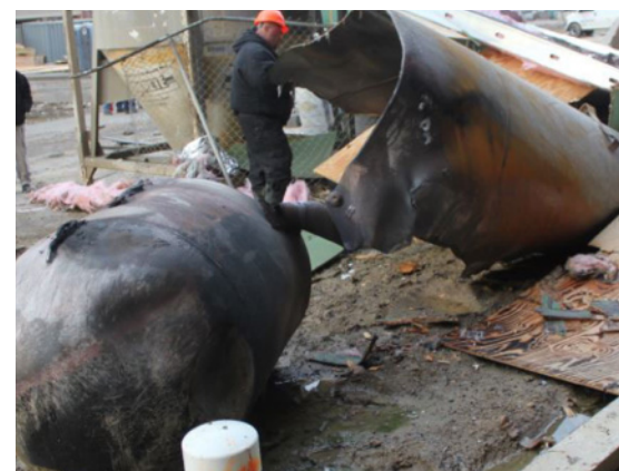
Container ruptured (BLEVED) from fire
